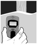
You can process joist detection now and please always press the power button during the detecting course.
